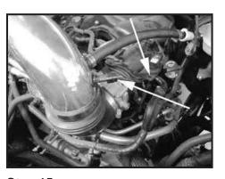
Step 15 Unclip the wiring harness from the mounting location. Now connect the IAT sensor by pushing the connector on the sensor.
