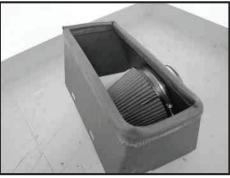
Step 8 Place the velocity stack adapter in the heat shield and install the supplied coupler making sure the coupler is pushed completely against the heat shield. Once the adapter and coupler are tight against the heat shield, tighten the clamp. Make sure that the clamp for the intake tube is installed but left loose at this time. Install the air filter and dress the heat shield with rubber seal.
