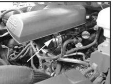
Step 3 Loosen the clamp on the tube going to the throttle body.
