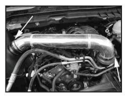
Step 13 Install the intake tube into the heat shield coupler and then into the coupler on the throttle body. Once in position fully tighten the clamps.
