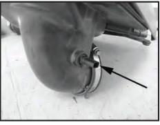
Step 10 Remove the IAT sensor from the factory intake tube.
