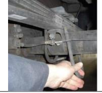
Remove u-bolts and carefully lower axle.
