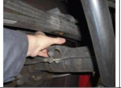
Center lift block on axle pad under leaf spring pin side down.
