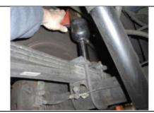
Work on one side of vehicle at a time, remove rear u-bolts.
