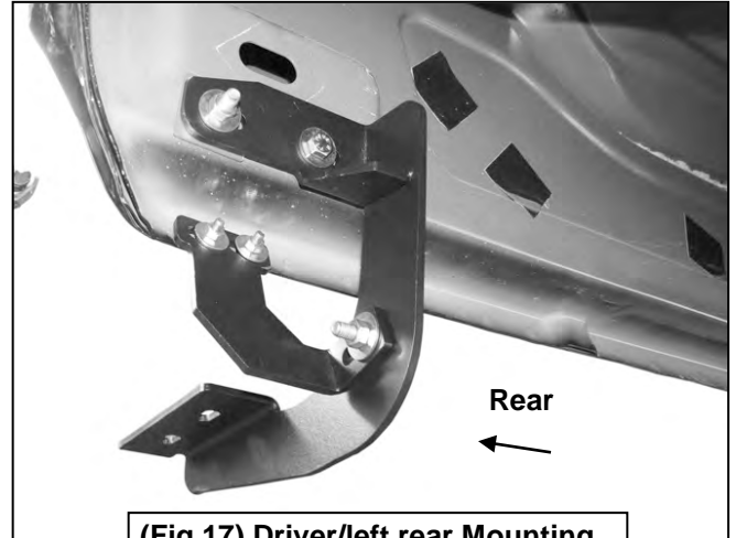
(Fig 17) Driver/left rear Mounting and Support Brackets
