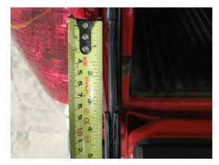
**Step 7\\** Install the cable clamp 3.5" below the upper cable end. This will prevent the cable from causing damage to the shock.
