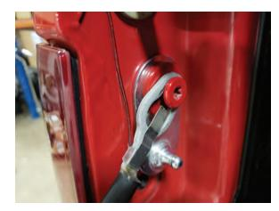
**Step 2\\** Install the upper bracket behind the upper lift gate bolt. Reinstall lift gate strap.
