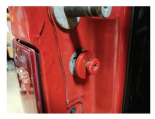
**Step 1\\** Remove the lift gate strap and loosen the T50 lift gate bolt.
