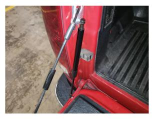
**Step 9**\\ Press the shock onto the ball stud mounts.
