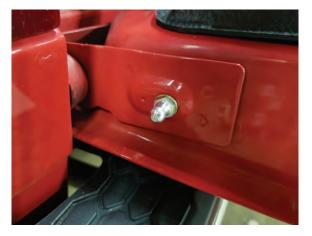
**Step 5\\** Apply blue thread lock to the threads of the ball mount. Torque the ball mount to 8ft-lbs.
