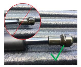
**Step 8\\** Before installing the shock ensure both of the shock ends are screwed on all the way.
