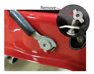
**Step 6\\** Loosen the lower cable mount. Remove the limiting washer as pictured.
