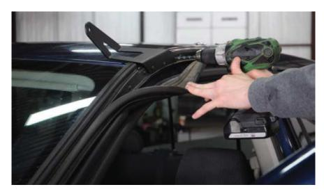
5. Using the supplied 3/16" rivets, rivet the bracket to the vehicle.
