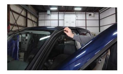
2. Remove the factory screw using a T15 Torx bit.
