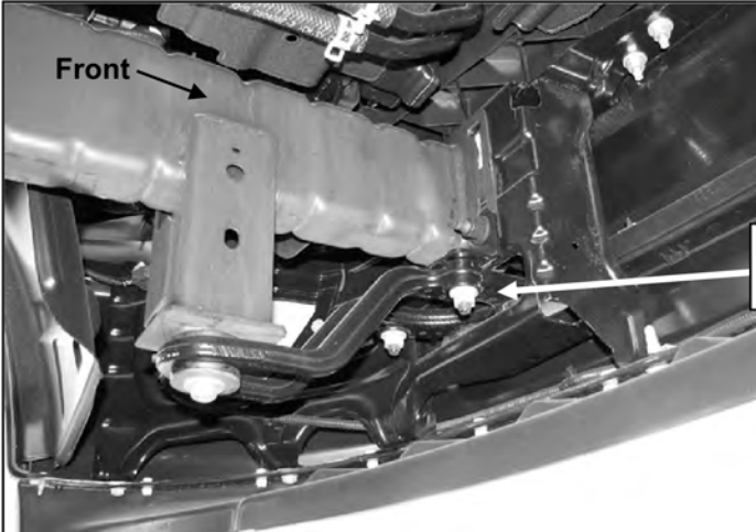
(Fig 6) Driver side mounting location pictured from behind bumper on tow hook equipped model
