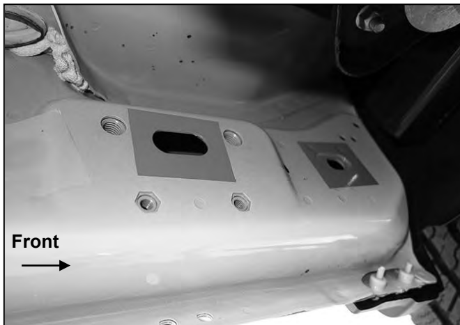
(Fig 8) Driver side front mid 2015-on, an example of models with factory installed threaded inserts
