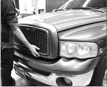
Step 1. Place supplied grille (A) onto the vehicle as shown.
