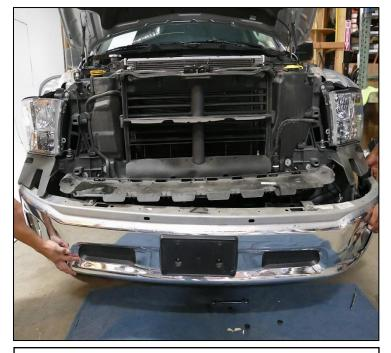
Step 2. With help from an assistant remove factory bumper from vehicle. Discard factory bumper.
