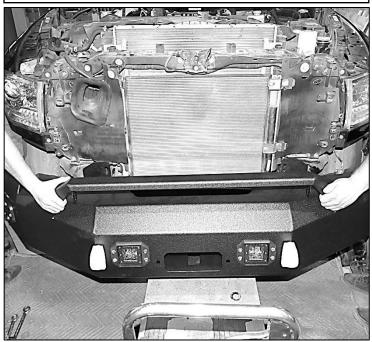
Step 3. With help from an assistant place new bumper (A) onto vehicle.
