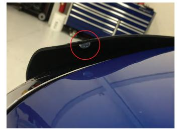
Step 2// Finish the installation by installing the supplied rubber bumpers to protect the paint anywhere the Bug Deflector may make contact with the hood.
