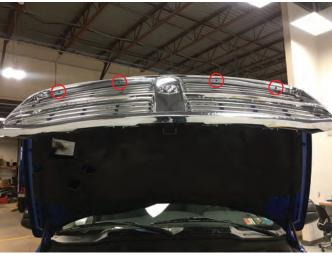
Step 1// Locate the (4) pre-existing holes on the factory grille. Align the bug deflector and install the (4) supplied plastic push clips.
