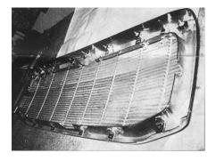
(3) Thread the #8 screws and flat nuts at each bracket. Re-install the grille shell assembly back onto the vehicle.
