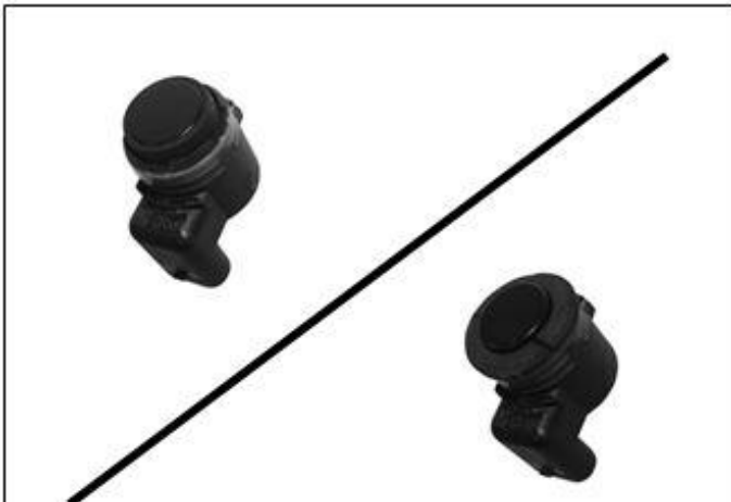
(Fig 10) Remove OE sensor washer and place the provided Foam Washer onto the front of the sensor
