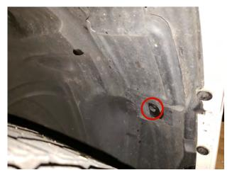
**STEP 3** // Located on the front wheel well liner, using a trim panel removal tool remove the (1) plastic push clip to gain access to the headlight retaining clip.
