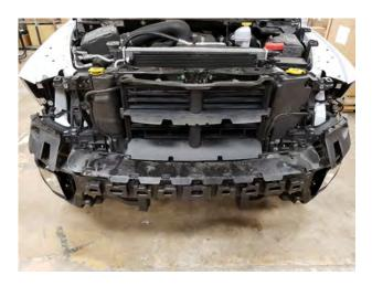
**STEP 9** // Carefully remove the bumper cover from the vehicle.
