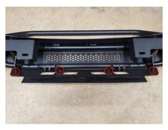
**STEP 17** // Install the mid plate to the bumper using the (4) M8x30mm allen bolts, (8) flat washers, (4) lock washers, and (4) nuts.
