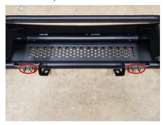
**STEP 15** // Install the (2) inner mid plate brackets with the optional (2) grille lightbar brackets using the (2) M8x30mm allen bolts, (4) flat washers, (2) lock washers, and (2) nuts. Repeat on each side.
