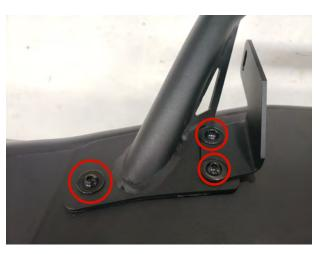
**STEP 14** // Install the optional overrider bar with the optional (2) lightbar mounts onto the bumper using the (3) M8x30mm allen bolts, (6) M8 flat washers, (3) M8 lock washers, and (3) M8 nuts. Repeat on opposite side. If choosing to not use the overrider bar, install the (2) overrider block off plates.
