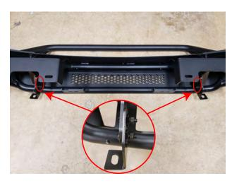
**STEP 16** // Install the (2) outer mid plate brackets using the (2) M8x30mm allen bolts, (4) flat washers, (2) lock washers, and (2) nuts. Repeat on each side.
