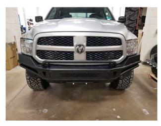
**STEP 19** // Install the bumper to the vehicle using the (6) M12x1.75x35mm bolts, flat washers, lock washers, and nuts. Be sure to center the bumper, and adjust height to desired location.
