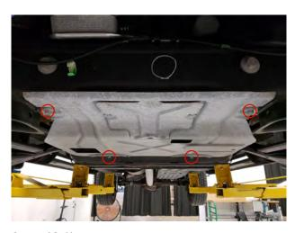
**STEP 13** // From underneath the vehicle, remove the (4) 15mm bolts securing the factory skid plate in place. Remove the skid plate.
