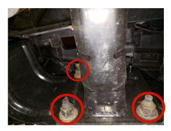
**STEP 10** // From underneath the vehicle, remove the (3) 18mm nuts on each side securing the bumper to the frame rail. Unplug the factory foglight harness, then remove the bumper from the vehicle.
