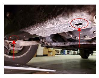
**STEP 21** // Hold the rear section of the skid plate in place to determine mounting location. Insert the (2) T-bolt plates into the radiator support. Insert the skid plate through the t-bolt, and secure using the flat washers, lock washers, and nuts.
