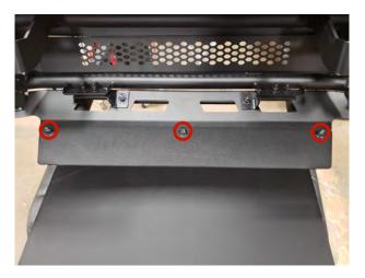
**STEP 18** // Attach the skid plate to the mid plate using (3) M8x30mm allen bolts, (6) M8 flat washers, (3) M8 lock washers, and (3) M8 nuts.
