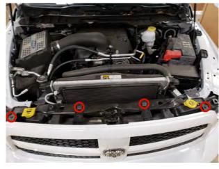
**STEP 2** // Next, remove the (4) 10mm bolts across the top of the factory grille. Then gently pry the grille away from the vehicle removing the grille.
