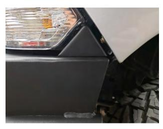
**STEP 20** // Install the (1) corner triangle to the bumper using (2) M6x1.0x20mm allen bolts, (2) flat washers, and (2) lock washers. Repeat on opposite side.
