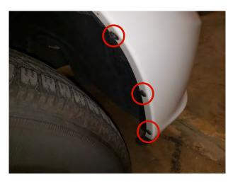
**STEP 7** // Using a 7mm socket & ratchet remove the screw securing the bumper cover to the fender liner. Then using a trim panel removal tool, remove the (2) plastic push clips. Repeat for the opposite side.
