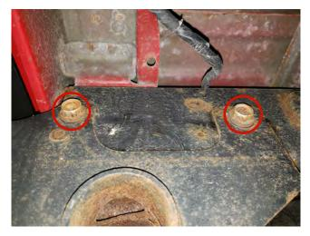
**STEP 3** // From underneath the vehicle, locate and remove the (2) 21mm bolts from the upper frame rail mount. Do the same on the opposite side. \*\*Note: Factory hardware will be reused.
