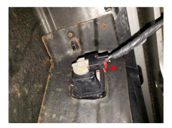
**STEP 2** // Push the red tab outwards, and press the black tab to unplug the license plate light harness. Unplug both sides.
