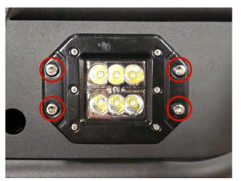
**STEP 7** // **Optional Light:** If choosing the LED fog light option, install the (2) LED Fog lights into the bumper using the (4) M6x1.0x15mm screws, lock washers, and nuts.
