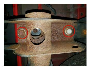
**STEP 4** // From under the vehicle, remove the (2) 21mm bolts from the lower frame rail mount. Do the same on the opposite side. Carefully remove the bumper from the vehicle. \*\*Note: Factory hardware will be reused.
