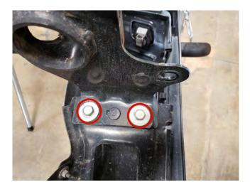
**STEP 10** // Remove the (2) 16mm bolts on each side securing the bumper mount to the factory rear bumper. Remove bumper mount.
