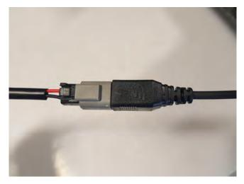
**STEP 14 // Optional Light Wiring:** Connect the (2) LED Fog lights into the supplied harness. Be sure to zip tie the access wiring away from any damage that could occur.
