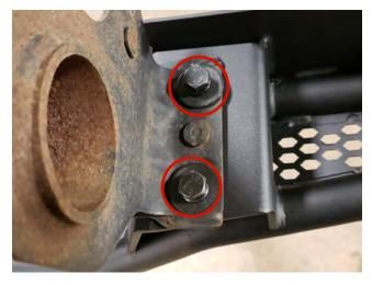
**STEP 11** // Attach the bumper mount to the new bumper using the (1) bolt plate, and (2) M12x1.75x40mm bolts, lock washers, and flat washers on each side.
