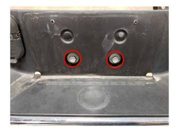
**STEP 9** // Located behind the license plate, remove the (2) 16mm bolts securing the center of the bumper mount to the bumper.
