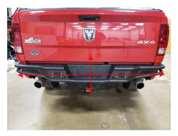
**STEP 12** // Attach the prerunner bumper to the vehicle using the factory hardware from Steps 3 & 4. Be sure to center the bumper, and adjust height of bumper to desired location. Then reinstall the trailer harnesses. If equipped, reinstall the backup camera harnesses.
