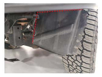
**STEP 17** // Remove / modify / secure the factory inner fender liners. Secure any and all factory components away from tire or suspension components. Installation is now complete.
