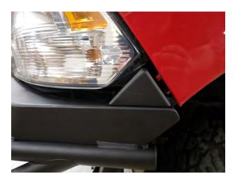
**STEP 16** // Install the (1) corner triangle to the bumper using (2) M6x1.0x20mm allen bolts, flat washers, and lock washers. Repeat on the opposite side. Reinstall grille and radiator plastic cover.
