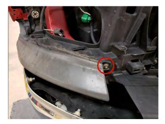
**STEP 11** // Located under the headlight, remove the (1) 10mm bolt on each side securing the bumper cover supports to the vehicle. Remove the supports.
