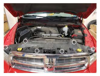
**STEP 1** // Open the hood. Locate and remove the (6) push clips using a trim panel removal tool. Remove radiator plastic cover from the vehicle.
