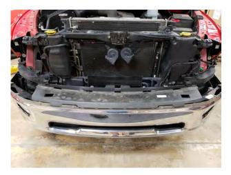
**STEP 8** // Carefully remove the bumper cover from the vehicle.
