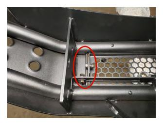
**STEP 13** // Insert the mesh bumper grille into the bumper. Secure the grille to the bumper using the (1) grille bracket, (2) M8x1.25x20mm bolts, flat washers, lock washers, and nuts. Repeat on the opposite side.
