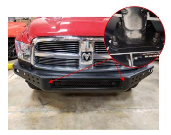
**STEP 15** // Install the bumper to the vehicle using the (8) M10x1.50x35mm bolts, flat washers, lock washers, and nuts. Be sure to center the bumper, and adjust height to desired location.
