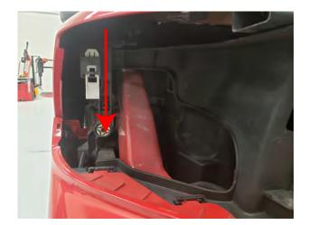
**STEP 4** // Gently reach into the access port and pull down on the headlight retaining clip. This will allow the headlight to be removed in a future step.
