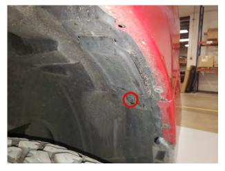
**STEP 3** // Located on the front wheel well liner, using a trim panel removal tool remove the (1) plastic push clip to gain access to the headlight retaining clip.
