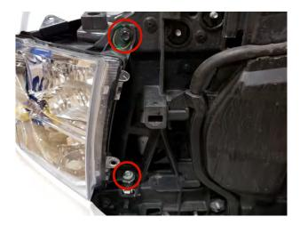
**STEP 5** // Locate, and remove the (2) 10mm bolts securing the headlight to the front support. Gently pull the headlight away from the vehicle. Unplug the headlight wire connectors, and remove the headlight from the vehicle.
