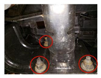
**STEP 10** // From underneath the vehicle, remove the (3) 18mm nuts on each side securing the bumper to the frame rail. Remove the bumper from the vehicle.
