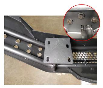
**STEP 14** // Install the bumper frame bracket to the bumper using (3) M12x1.75x35mm bolts, flat washers, lock washers, and nuts. Repeat on the opposite side.
