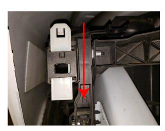
**STEP 4** // Gently reach into the access port and pull down on the headlight retaining clip. This will allow the headlight to be removed in a future step.
