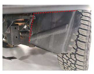
**STEP 17** // Remove / modify / secure the factory inner fender liners. Secure any and all factory components away from tire or suspension components. Installation is now complete.
