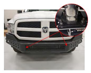
**STEP 15** // Install the bumper to the vehicle using the (6) M12x1.75x35mm bolts and (2) M10x1.5x45mm bolts, flat washers, lock washers, and nuts. Be sure to center the bumper, and adjust height to desired location.
