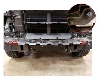
**STEP 12** // Remove the (4) 10mm bolts securing the center support to the vehicle. Remove the center support.
