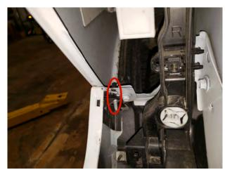
**STEP 6** // Inside the headlight bucket, locate and remove the (1) 10mm bolt on each side securing the bumper cover to the fender.
