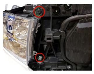
**STEP 5** // Locate, and remove the (2) 10mm bolts securing the headlight to the front support. Gently pull the headlight away from the vehicle. Unplug the headlight wire connectors, and remove the headlight from the vehicle.
