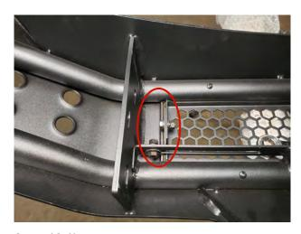
**STEP 13** // Insert the mesh bumper grille into the bumper. Secure the grille to the bumper using the (1) grille bracket, (2) M8x1.25x20mm bolts, flat washers, lock washers, and nuts. Repeat on the opposite side.
