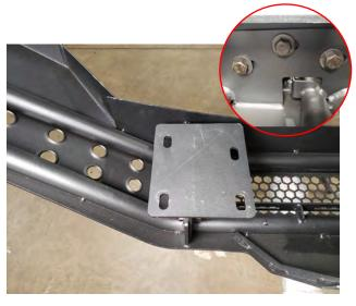
**STEP 14** // Install the bumper frame bracket to the bumper using (3) M12x1.75x45mm bolts, flat washers, lock washers, and nuts. Repeat on the opposite side.
