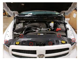
**STEP 1** // Open the hood. Locate and remove the (6) push clips using a trim panel removal tool. Remove radiator plastic cover from the vehicle.
