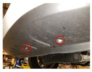
**STEP 8** // From underneath the vehicle, remove the (2) 13mm bolts securing the bumper cover to the bumper.
