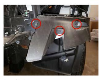
**STEP 11** // Located under the headlight, remove the (3) 10mm bolts on each side securing the bumper cover supports to the vehicle. Remove the supports.
