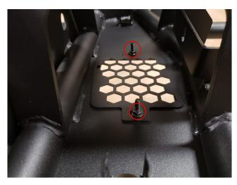
**STEP 8** // If choosing not to use the LED fog lights, install the (2) mesh grille inserts into the bumper using the (2) M6 flat washers, lock washers, and nuts.
