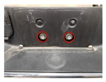
**STEP 9** // Located behind the license plate, remove the (2) 16mm bolts securing the center of the bumper mount to the bumper.
