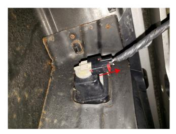
**STEP 2** // Push the red tab outwards, and press the black tab to unplug the license plate light harness. Unplug both sides.
