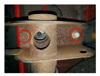
**STEP 4** // From under the vehicle, remove the (2) 21mm bolts from the lower frame rail mount. Do the same on the opposite side. Carefully remove the bumper from the vehicle. \*\*Note: Factory hardware will be reused.
