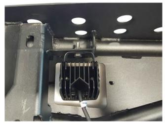
**STEP 7** // **Optional Light:** If choosing the LED fog light option, install the (2) LED Fog lights into the bumper using the (2) M8x1.25x30mm bolts, flat washers, lock washers, and nuts.
