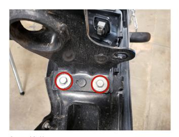
**STEP 10** // Remove the (2) 16mm bolts on each side securing the bumper mount to the factory rear bumper. Remove bumper mount.
