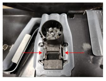
**STEP 5** // Using a flat head screw driver, push in the metal tabs on the trailer plug connector and remove from the factory bumper. Transfer to new bumper.
