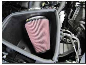
16. Install the K&N<sup>®</sup> air filter onto the filter adapter and secure with the provided hose clamp.
