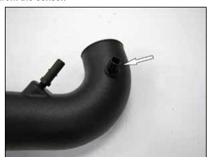
13. Install the sensor into the K&N<sup>®</sup> intake tube using the provided grommet.
