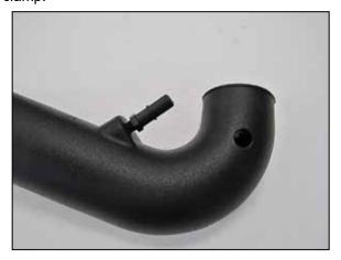
11. Install the provided NPT quick disconnect fitting into the  $K\&N^{\mbox{\scriptsize @}}$  intake tube as shown.
