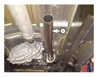
Fasten inlet with (x2 ea) bolts (13), flat washers (15), lock washers (16) and nuts (14). Place clamp (12) onto extension (2) and connect it to inlet pipe. Insert hanger in isolator, tighten clamp and reclip ground wire.
