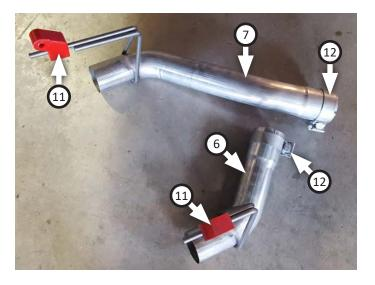
14. Connect right and left rear tailpipes to front tailpipes, then rotate them and to insert hangers. Tighten clamps just enough to allow for later adjustment.
