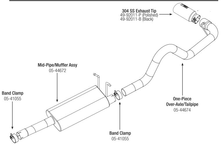
**Step 1: (Read Instructions prior to installation)** Remove your stock exhaust from the rear of your truck working your way forward. It may be necessary to cut the pipes if the slip joints are stuck. Do not cut the pipe after the cat. You will be using this slip connection. Take caution not to damage the factory isolation mounts, as they will be reused. It is recommended to not fully tighten the clamps until the entire system is installed.
