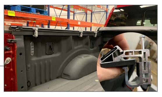
Evenly space (3) of the supplied bed rail clamps along each side of the bed. The clamp will engage the factory bed rail and the tonneau cover rail. Do not fully tighten these at this time.
