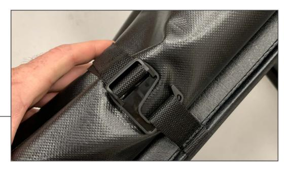
Fold the tonneau cover back when not in use. Secure the tonneau cover to the using the attached nylon strap and hook. Installation is now complete.
