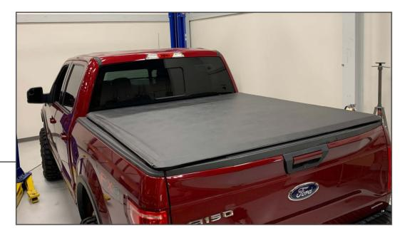
With the tonneau cover installed, loosen and re-position as needed for best fit. Tighten all clamps once the tonneau cover is in its final position.
