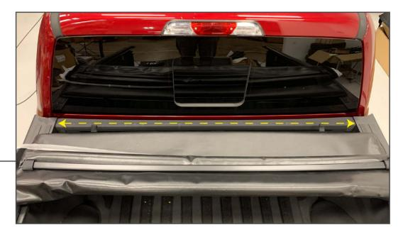
For vehicles with factory bed rails that sit higher than the front edge of the bed, apply the supplied weather strip to fill the gap. This will help reduce water intrusion. For vehicles where there front edge is flush with the bed rails this step is not required.
