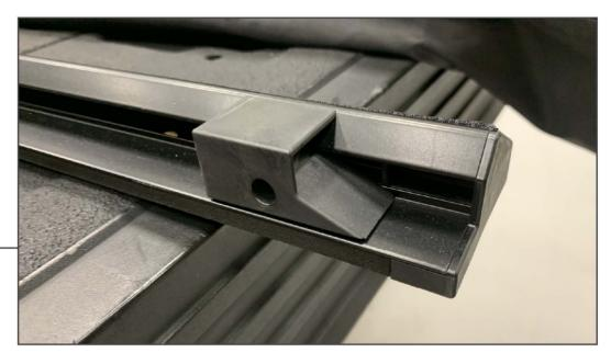
Position the tonneau cover rails on the vehicle. The hook and loop will face away from the bed. The end with the black plastic cap/latch faces the rear of the vehicle.
