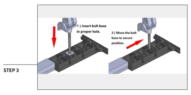
Insert the clamping bolt into the threaded insert. Move the bolt and threaded insert to the appropriate mounting location.
