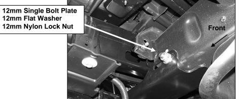
(Fig 11) Passenger Bracket installed in "forward" position to move Bull Bar away from bumper
