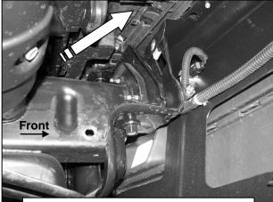
(Fig 2) 2014-15 models, from behind the bumper, remove the clips securing the facia to the top of the bumper
