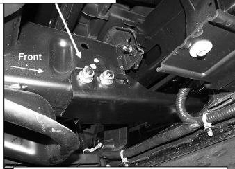
(Fig 9) Note Bracket installed in "forward" position to move Bull Bar away from bumper
