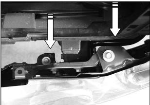
(Fig 3) 2016 model to show bumper bolt locations from above (arrows) with grille removed. 2014-15 models also remove plastic facia panel to access bumper bolts as necessary
