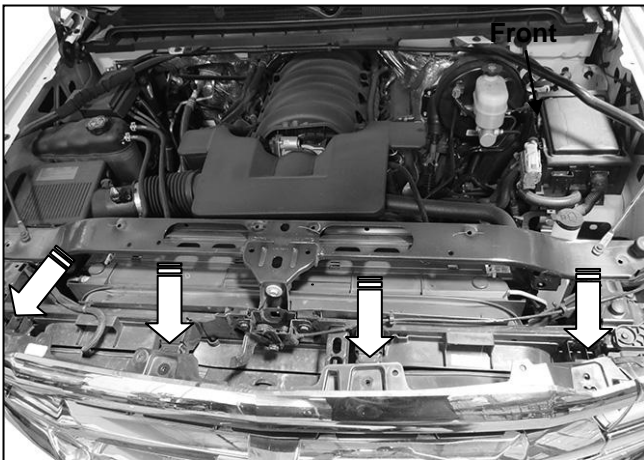
(Fig 1) Remove cover between radiator and grille. Remove screws attaching top of grille (arrows)
