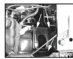
Step 6 Remove the air box mounting plate. Three of these bolts will be re installed with the new heat shield.
