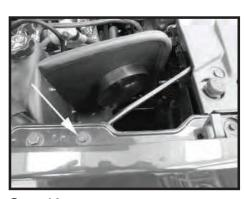
Step 12 Remove the bolt shown and rotate the brace towards the engine.
