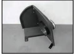
Step 9 Assemble the heat shield with the tabs placed on the outside of heat shield. Install the rubber bulb seal. Place the velocity stack adapter in the heat shield and install the supplied flex coupler making sure the coupler is pushed completely against the heat shield. Take note of the orientation of the funnel, this may be rotated slightly once the filter is installed in the vehicle. Once the adapter and coupler are tight against the heat shield, tighten the clamp.
