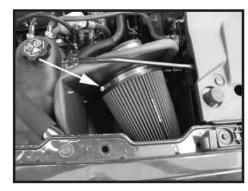
Step 13 Install the filt the clamp.
