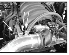
Step 17 Connect the supplied hose to the breather tube on the motor. Install the new hose onto the vacuum fitting on the intake tube.
