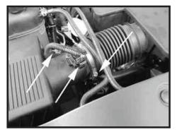
Step 2 Loosen the clamp at the air box. **Disconnect the Mass Air Flow** Sensor (MAFS) electrical connector and unclip the wiring harness from the air box.
