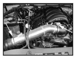
Step 16 Install the intake tube as shown and once in position tighten clamps.
