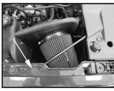
Step 14 Reinstall the bolt that was removed in Step 12.
