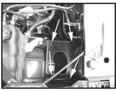
Step 6 Remove the air box mounting plate. Three of these bolts will be re installed with the new heat shield.
