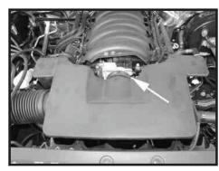
Step 4 Loosen the clamp at the throttle body and remove the factory plenum from the vehicle.
