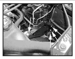
Step 11 This step is only required if your heat shield bolt pattern did not line up in Step 10. Loosen the 4 bolts shown, but do not remove them. Install the heat shield and fasten it securely in place. Once the heat shield is in place, securely fasten the 4 bolts that were just loosened.
