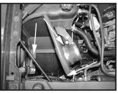
Step 10 Install the heat shield into the truck as shown by reusing the hardware from the tray removed in Step 6. If the holes do not line up with the heat shield, see the next step to resolve this.
