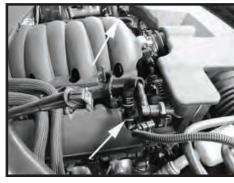
Step 3 Disconnect the breather tubes from the engine. There is a small tab on the end of the tube, push it to release the breather tube.
