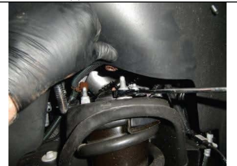
Loosen upper strut mount bolts
