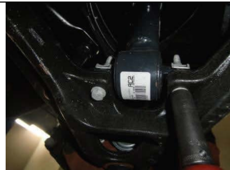
Remove lower strut mounting bolts
