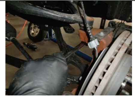
Loosen upper ball joint nut and leave attached.
