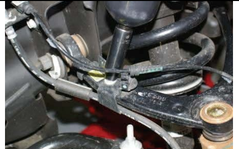
Disconnect ABS/brake bracket from upper control arm.
