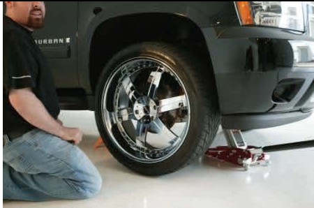
Raise and support front of vehicle frame on jack stands
