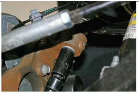
Tighten upper ball joint to spec.
