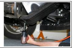
2. With the vehicle on level ground, set the emergency brake and block the rear tires. Jack up the front end of the truck and support the frame rails with jack stands. **NEVER WORK UNDER AN UNSUP-PORTED VEHICLE!** Remove the front wheels.
