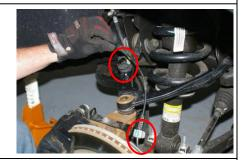
4. A 10mm socket is used to remove the brake line bracket that attaches to the upper control arm.
