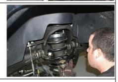
14. Place a jack under the lower control arm and raise it up. Then place the new ReadyLift lower strut mount spacer over the factory control arm holes as shown.
