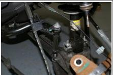
18. Using a pry bar inserted through the coil spring and over the upper control arm, pry downward to force the control arm down and the ball joint stem into the spindle. Install the factory nut and tighten.
