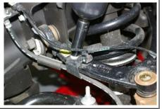
5. An 18mm socket is used to loosen the upper ball joint nut. The nut should remain on the ball joint stem.
