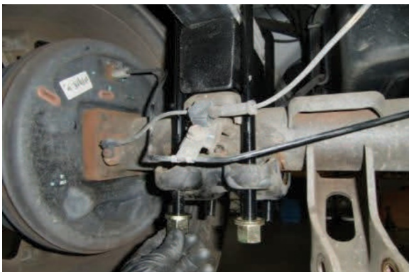
Install new, longer, U-bolts and hardware.
