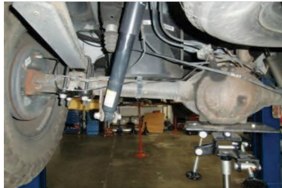
Support the rear axle with a jack.
