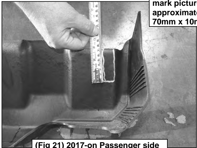
(Fig 21) 2017-on Passenger side DEF cover marked for trimming
