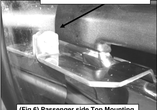
(Fig 6) Passenger side Top Mounting Bracket installation pictured
