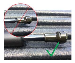
**Step 6\\** Before installing the shock ensure both of the shock ends are screwed on all the way.
