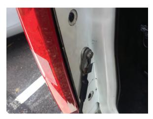
**Step 1\\** Remove the lift gate strap and loosen the 13mm lift gate bolt.
