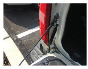
**Step 7\\** Press the shock onto the ball stud mounts.
