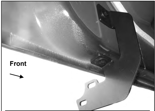
(Fig 10) Driver/left side rear Bracket installed
