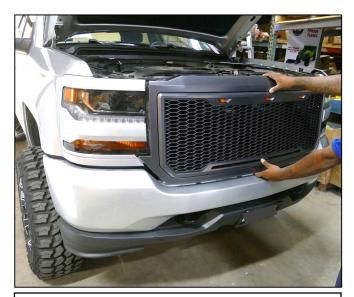
Step 1 Place supplied grille (A) onto vehicle as shown.
