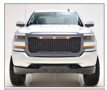
Step 2 Install grille (A) onto vehicle by reversing steps 1-2 in page 2.
