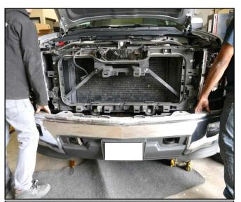
Step 11 With help from an assistant remove factory bumper from vehicle. Set factory bumper aside in a protected area.
