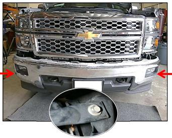
Step 8 Working underneath the vehicle. Using a 15mm socket locate and remove the two bolts mounted onto the side of the bumper as shown. Discard factory hardware.
