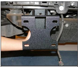
Step 1 Locate and place supplied mounting bracket (B) onto vehicle. Line up the holes in the mounting bracket with the holes in the vehicle frame.
