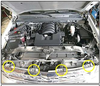
Step 2 Using a 10mm socket locate and remove 4 factory bolts securing factory grille onto vehicle. Set hardware aside for reinstallation.
