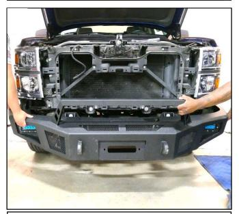
Step 1 With help from an assistant place supplied bumper (A) onto vehicle. Line up the bumper the holes with the holes in the mounting bracket.
