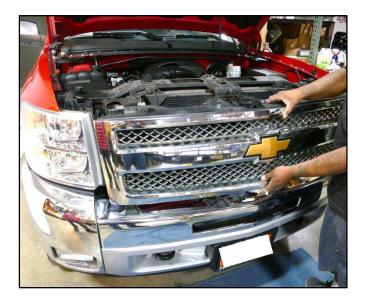
Step 3 Firmly grab and pull factory grille off of vehicle. Place factory grille aside for later use.
