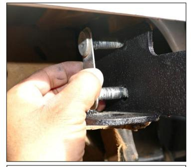
Step 2. Install factory hardware removed in step 2 (removal process) through the holes in the mounting bracket (C) and through the holes in the vehicles frame.
