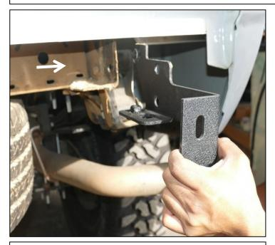
Step 1. Install passenger mounting bracket (C) onto vehicle as shown.
