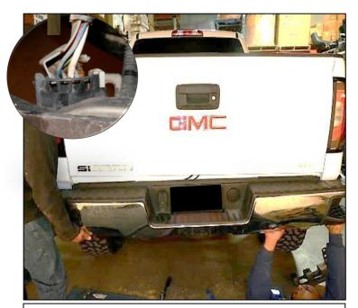
Step 5. Locate and remove the locking clip to unplug the trailer harness. With help from an assistant push down on factory bumper and remove bumper from vehicle.
