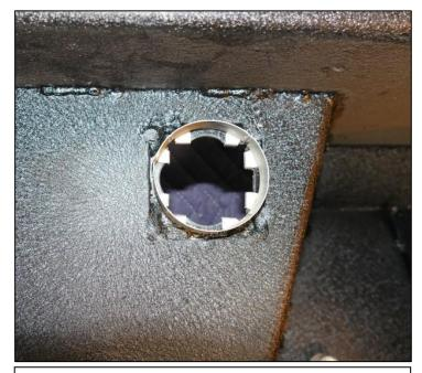
Step 3. Working behind the bumper. Place outer ring onto bumper as shown.
