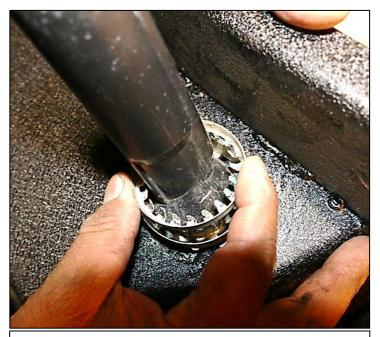
Step 5. Working behind supplied bumper (A). Install inner ring into outer ring as shown above to secure spare tire access housing onto supplied bumper (A).
