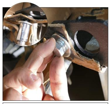
Step 4. Working underneath mounting bracket. Locate and place supplied hex head bolt M12x1.75 40mm (D) with M12 split washer (F) and flat washer (G) onto mounting bracket. Tighten down using 18mm socket.
