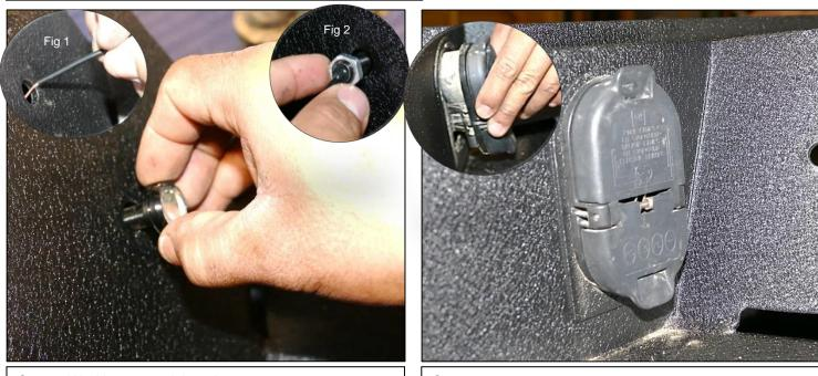
Step 1. Working on work bench. Feed supplied LED marker (H) cable through license plate light hole fig 1. Start supplied nut at the end of light shown in fig 2. Finger tighten only. Repeat step for other side LED light.
