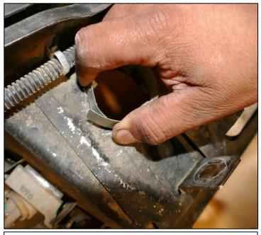
Step 7. Remove outer ring by pressing firmly on all side of the outer ring. Set outer ring aside for reinstallation.
