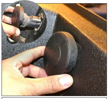
Step 4. Install spare tire access into bumper.
