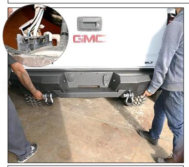
Step 6. With help from an assistant place supplied rear bumper (A) onto vehicle. Reinstall the hitch receiver locking clip onto hitch harness. Line up bumper holes with mounting bracket holes.
