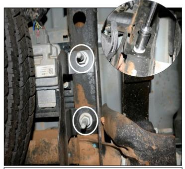
Step 4. Using a 21mm deep socket locate and remove two factory bolt holding factory tow hitch onto vehicle. Repeat for other side. With help from an assistant remove factory hitch from vehicle. Set hardware and factory tow hitch aside for reinstallation.
