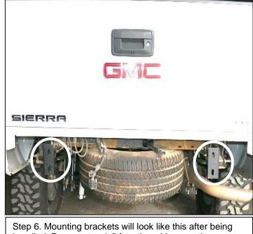
Step 6. Mounting brackets will look like this after being installed. Repeat step 1-5 for other side mounting bracket.
