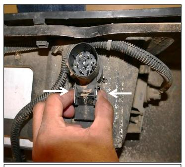
Step 8. Locate and remove hitch harness by firmly pressing on both clips as shown. Remove hitch harness from factory bumper. Set hitch harness aside for later use.
