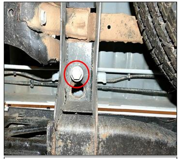
Step 3. Using a 21mm socket locate and remove factory bolt holding factory hitch onto vehicle. Repeat for other side. Set hardware aside for reinstallation.
