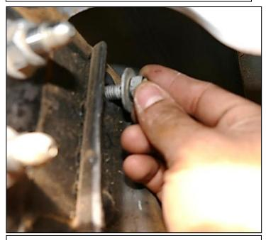
Step 5. Install factory bolt removed in step 2 (removal process) through vehicle frame holes onto mounting bracket (C). Using a 15mm socket tighten down bolt.
