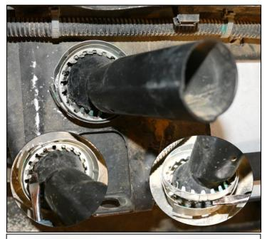
Step 6. Proceed to your work bench. Working behind bumper locate and remove middle ring holding spare tire access housing onto bumper using a flat head screwdriver. Remove spare tire access housing. Set middle ring and spare tire access housing aside for later use.
