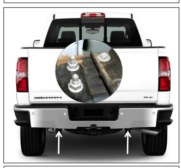
Step 1. Working underneath the vehicle. On each side of the bumper you will need to locate 3 factory bolts.
