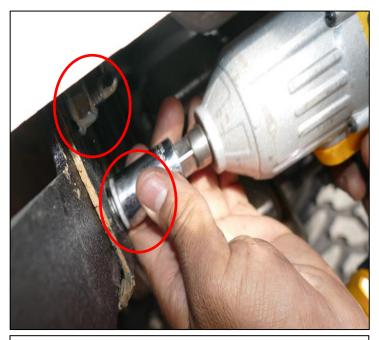
Step 3. Start factory nuts at the end of the bolts. Using a 19mm socket (or impact wrench) tighten down nuts.
