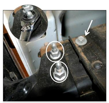
Step 2. Using a 19mm socket locate and remove 2 factory nuts circled above. Remove top right bolt using a 15mm socket. Repeat step for other side. Set factory hardware aside for reinstallation.
