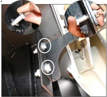
Step 7. Locate and place supplied hex head bolt 12x1.75 40mm (D) with supplied flat washer M12 (G) from behind mounting bracket holes and through the bumper (A) holes fig 1. Start a supplied hex head bolt M12 (E) at the end of bolt. Tighten down using 18mm socket. Repeat step for remaining bolt. Repeat same step for other side of bumper.
