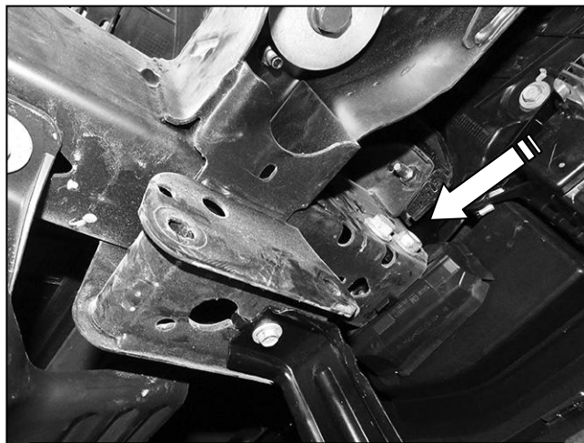
(Fig 3) Passenger/right outer mounting bolts for tow hook pictured from behind bumper
