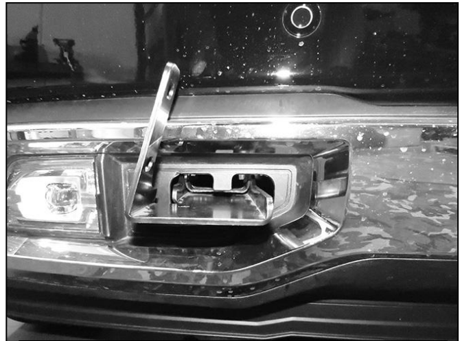
(Fig 11) Passenger/right side Bracket installed
