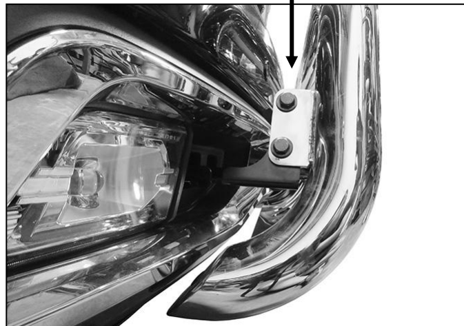
(Fig 13) Passenger/right side complete installation
