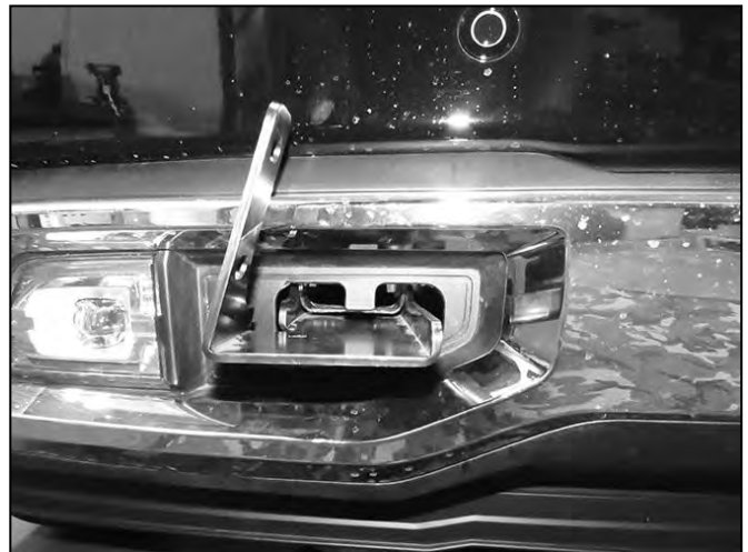
(Fig 11) Passenger/right side Bracket installed
