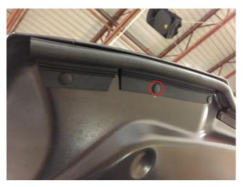
Using a panel removal tool or a flat head screw driver, remove those (6) push pins.
