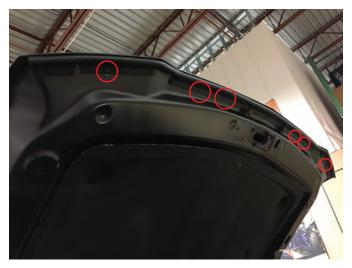
Step 1// Open hood and center the Bug Deflector to the hood. This will allow you to identify which of the (6) factory push pins need to be removed. \*\*Note: the factory push pins will not be reused.
