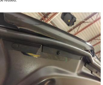
Step 3// Once the factory push pins are removed, sandwich the bug deflector between the weather-stripping and the hood. Install the supplied push pins. \*\*Note: These are a tight fit and will require you to apply firm pressure on the supplied push pin to insure they are pin catches the weather stripping, Bug Deflector, and the hood.
