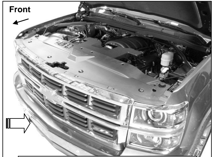
(Fig 1) Unplug sensors, fog lights and move wiring harness away from bumper before removal
