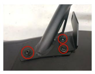
**STEP 11** // Install the optional overrider bar with the optional (2) lightbar mounts onto the bumper using the (3) M8x30mm allen bolts, (6) M8 flat washers, (3) M8 lock washers, and (3) M8 nuts. Repeat on opposite side. If choosing to not use the overrider bar, install the (2) overrider block off plates.
