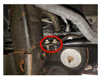
**STEP 6** // From underneath the vehicle, locate and remove the (2) 15mm bolts on each side securing the side bumper brackets to the frame. Carefully remove the bumper from the vehicle.
