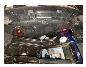
**STEP 9** // Below the headlight, remove the (2) 10mm bolts on each side securing the bumper cover stiffeners. Remove both stiffeners.
