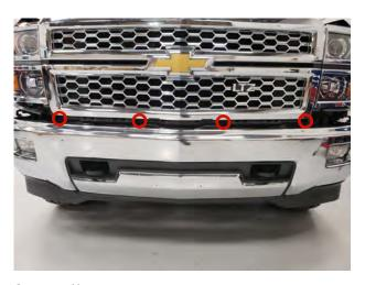
**STEP 4** // Remove the lower (4) 10mm grille bolts. Gently pry the grille away from the vehicle, and remove the grille.
