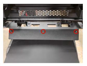
**STEP 14** // Attach the skid plate to the mid plate using (3) M8x25 allen bolts, (6) flat washers, (3) lock washers, and (3) nuts.
