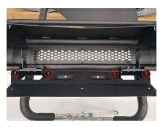
**STEP 13** // Install the mid plate to the bumper using the (4) M8x25mm allen bolts, (8) flat washers, (4) lock washers, and (4) nuts.
