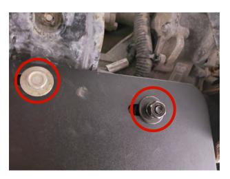
**STEP 16** // Install the skid plate to the radiator support using a 15mm bolt from Step 10 and (1) M10x30mm T bolt, flat washer, lock washer, and nut. Reinstall the factory grille.
