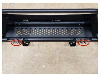
**STEP 12** // Install the (2) mid plate brackets with the optional (2) grille lightbar brackets using the (4) M8x30mm allen bolts, (8) flat washers, (4) lock washers, and (4) nuts.
