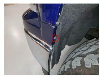
**STEP 3** // Locate, and remove the 8mm screw on each side of the bumper cover. Gently pry the bumper cover away from the vehicle to remove.
