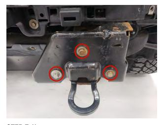
**STEP 7** // Remove the (3) 18mm bolts on each side securing the bumper brackets to the frame rail. \*\*Note: The hardware will be used to mount the new bumper.
