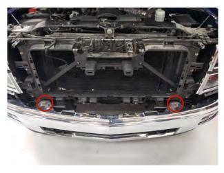
**STEP 5** // Locate, and remove the (2) 18mm bolts holding the upper portion of the bumper to the frame.
