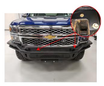
**STEP 15** // Install the bumper to the vehicle using the factory hardware from Step 7. Be sure to center the bumper, and adjust height to desired location.
