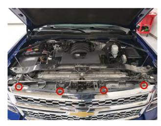
**STEP 2** // Next, remove the (4) 10mm bolts across the top of the factory grille.
