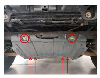
**STEP 10** // Locate, and remove the (6) 15mm bolts securing the factory skid plate. Remove skid plate.
