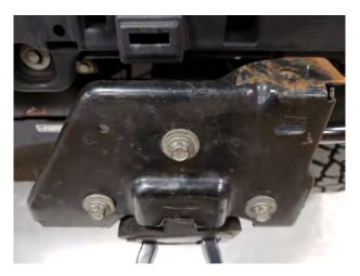
**STEP 5** // Locate, and remove the (2) 18mm bolts holding on the bumper frame brackets. Remove the brackets.
