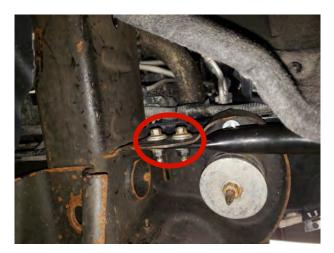
**STEP 12** // Remove the (2) 15mm bolts securing the factory side bumper bracket. Remove the bracket. Do the same for the opposite side. \*\*Note: These will not be reused.
