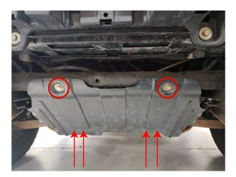
**STEP 11** // Locate, and remove the (6) 15mm bolts securing the factory skid plate. Remove skid plate.
