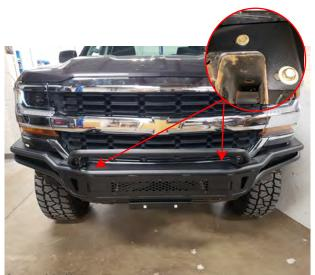
**STEP 13** // Install the bumper to the vehicle using the factory hardware from Step 5. Be sure to center the bumper, and adjust height to desired location.
