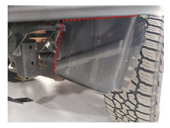
**STEP 15** // Remove / modify / secure the factory inner fender liners. Secure any and all factory components away from tire or suspension components. Installation is now complete.
