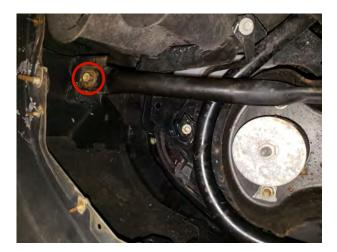
**STEP 4** // From underneath the vehicle, locate and remove the (1) 15mm bolt on each bumper side bracket. Carefully remove the bumper from the vehicle.
