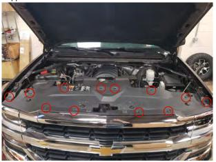
**STEP 1** // Open the hood. Locate and remove the (12) push clips using a trim panel removal tool. Remove radiator plastic cover from the vehicle.
