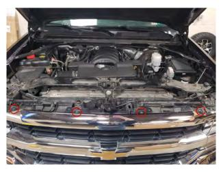
**STEP 2** // Next, remove the (4) 10mm bolts across the top of the factory grille. Gently pry the grille away from the vehicle, and remove the grille.
