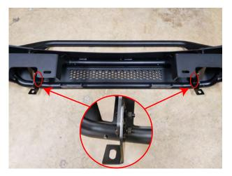
**STEP 8** // Install the (2) outer mid plate brackets using the (2) M8x30 allen bolts, (4) flat washers, (2) lock washers, and (2) nuts. Repeat on each side.
