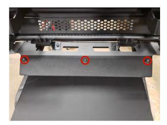
**STEP 10** // Attach the skid plate to the mid plate using (3) M8x30 allen bolts, (6) M8 flat washers, (3) M8 lock washers, and (3) M8 nuts.
