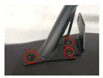
**STEP 6** // Install the optional overrider bar with the optional (2) lightbar mounts onto the bumper using the (3) M8x30mm allen bolts, (6) M8 flat washers, (3) M8 lock washers, and (3) M8 nuts. Repeat on opposite side. If choosing to not use the overrider bar, install the (2) overrider block off plates.
