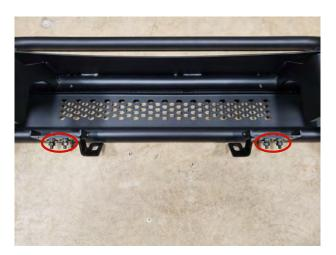
**STEP 7** // Install the (2) inner mid plate brackets with the optional (2) grille lightbar brackets using the (2) M8x30 allen bolts, (4) flat washers, (2) lock washers, and (2) nuts. Repeat on each side.
