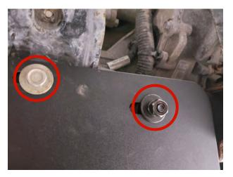
**STEP 14** // Install the skid plate to the radiator support using the (2) 15mm factory bolts from Step 11. Reinstall the factory grille.
