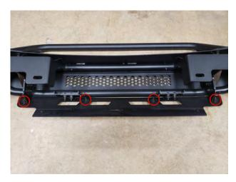
**STEP 9** // Install the mid plate to the bumper using the (2) M8x30 allen bolts, (4) flat washers, (2) lock washers, and (2) nuts. Repeat on each side.
