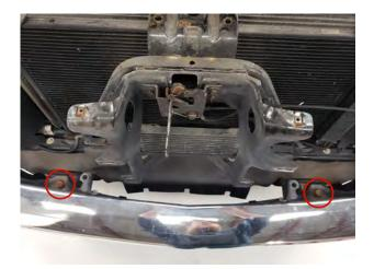
**STEP 3** // Locate, and remove the (2) 18mm bolts holding the upper portion of the factory bumper to the frame rail.
