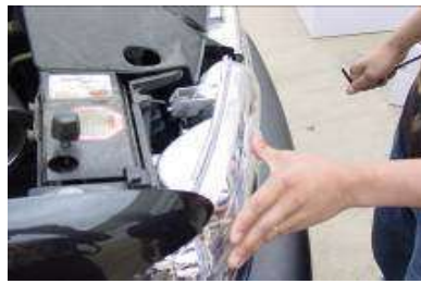
Step 10: Put the headlight back into the housing and use the pins to lock in the headlight.
