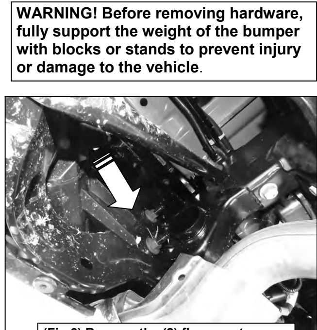
(Fig 6) Remove the (2) flange nuts per side attaching the bumper to the frame
