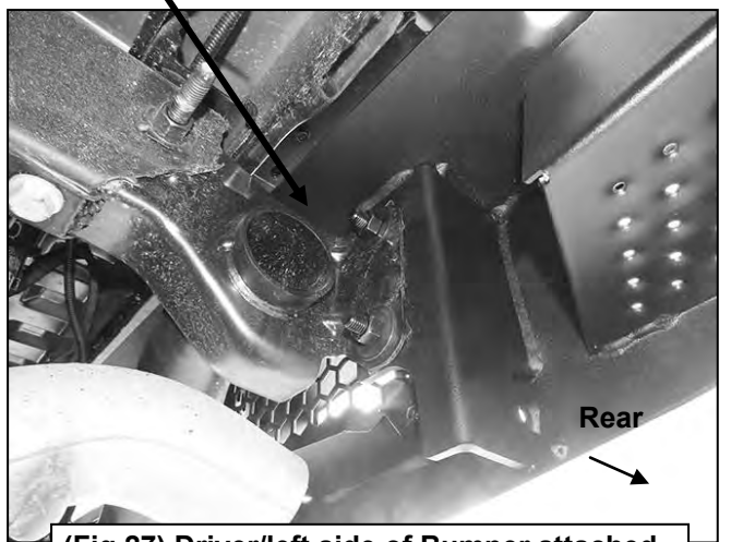
(Fig 27) Driver/left side of Bumper attached to the frame and Double Bolt Plate
