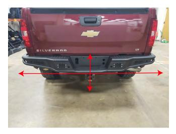
**STEP 12** // Attach the prerunner bumper to the bumper brackets using the (4) M12x1.75x40mm bolts, flat washers, lock washers, and nuts. Be sure to center the bumper, and adjust height of bumper to desired location. Then reinstall the trailer harnesses. If equipped, reinstall the backup camera harnesses.
