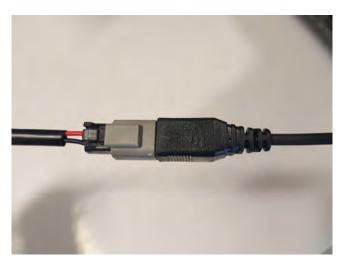
**STEP 14** // **Optional Light Wiring:** Connect the (2) LED Fog lights into the supplied harness. Be sure to zip tie the access wiring away from any damage that could occur.
