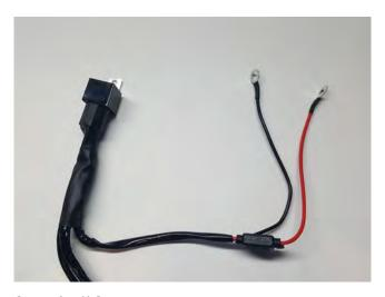
**STEP 15** // **Optional Light Wiring:** Install the Red 12+volt wire to the positive battery terminal. Connect the Black ground wire to the negative battery terminal. Mount the fuse in a safe location away from any damage that could occur. Tuck away any extra wiring.
