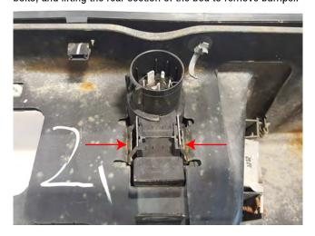
STEP 4 // 2014 + Silverado's, using a flat head screw driver, push in the metal tabs around the trailer plug connector and remove it from the factory bumper. Transfer to new bumper.
