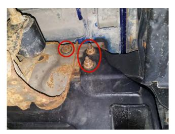
STEP 3 // Remove the (2) 18mm nuts, double bolt plate, and the (1) 15mm bolt on each side that holds the bumper to the top frame rail. Remove bumper from vehicle. \*\*Note: 2014+ Silverado's require loosening the (2) 21mm rear body to bed bolts, and lifting the rear section of the bed to remove bumper.
