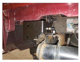
**STEP 11** // Attach the bumper bracket to the frame rail using (2) M14x2.0x45mm bolts, washers, and lock nuts, and (1) M10x1.50x50mm bolt, washers, and lock nut. Repeat on the opposite side.
