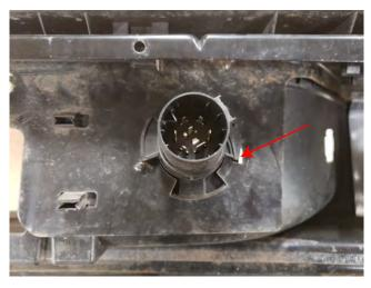
**STEP 5** // 2007-2013 Silverado's, using a flat head screw driver, lift up on the plastic tab on the trailer plug connector and twist the connector counter-clockwise to remove from the factory bumper. Transfer to new bumper.
