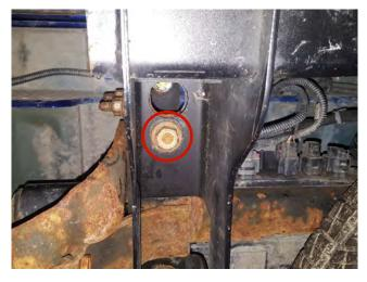
**STEP 2** // From under the vehicle, remove the (1) 21mm bolt on each side that holds the bumper to the bottom frame support.
