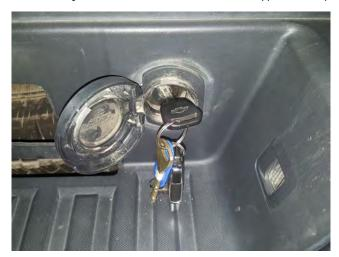
**STEP 7** // Using your factory ignition key, turn the spare tire lock clockwise and remove the spare tire lock from the factory bumper. Transfer to the new bumper.
