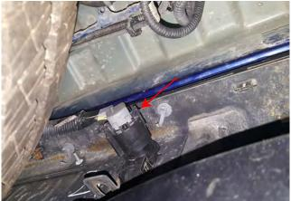
**STEP 1** // Unplug the factory license plate light harnesses, and the trailer plug connector and pull away from the bumper. If equipped unplug and remove the factory backup sensors.
