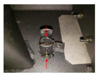
**STEP 6** // If equipped re-install the factory reverse sensors w/ the rubber grommet flush to the outer face of the bumper. \*\*Note: The factory trim bezel does not get re-used. Using the supplied 4mm screws to apply slight pressure to either side of the sensor. Over tightening of the screws can cause sensor damage. For vehicles w/o sensors install the supplied rubber plugs.
