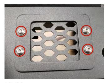
**STEP 8** // If choosing not to use the LED fog lights, install the (2) mesh grille inserts into the bumper using the (4) M6x1.0x15mm screws, lock washers, and nuts.
