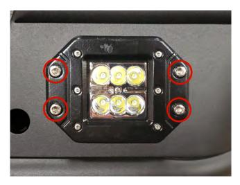
**STEP 9** // **Optional Light:** If choosing the LED fog light option, install the (2) LED Fog lights into the bumper using the (4) M6x1.0x15mm screws, lock washers, and nuts.
