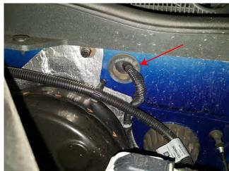
**STEP 16** // **Optional Light Wiring:** Route the on/off switch to the interior of the vehicle using a suitable body grommet. Mount the switch in the desired location. Zip tie any extra loose wiring away from any damage that could occur. Installation is now complete.
