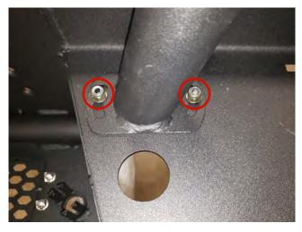
**STEP 10** // Install the spare tire guide bracket to the bumper using the (2) M6x1.0x20mm allen bolts, (4) M6 flat washers, and (2) M6 lock nuts.
