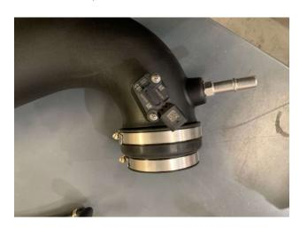
**STEP 35**Attach the MAF Harness Extension Cable (8) to the MAF sensor.
