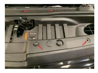
Disconnect and remove the support brace.
