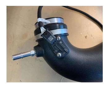
Snap-in a Push-In Cable Tie (26) into the insert on the back of the intake tube. Loop the cable tie into itself and feed the MAF Harness Extension Cable through it
