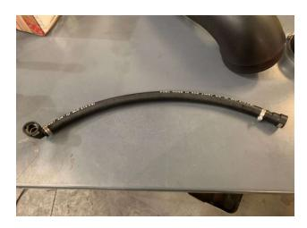
Install the Hose Assembly from Step 39. Install the straight end connector to the engine and right-angle connector to the intake tube
