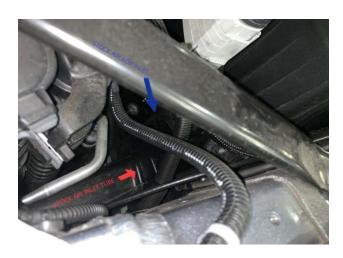
Carefully disconnect the large wire harness at the front of the air intake. The snap feature is designed to release under sufficient upward force; however, pulling and tilting the harness toward the rear of the vehicle will typically help disconnect the harness.
