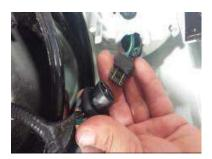
Next plug the connectors into your stock socket. Be sure to line the black wire up on the same side on both the socket and connector.
