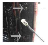
Remove the 2 Torx screw holding the taillight in.
